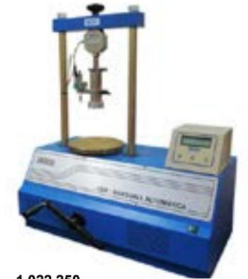
1.022.250 - Prensa CBR / Marshall Digital Microprocessada
